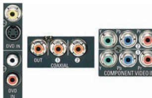
Figure 22 – DVD AV, Digital Audio and Component Video Inputs
